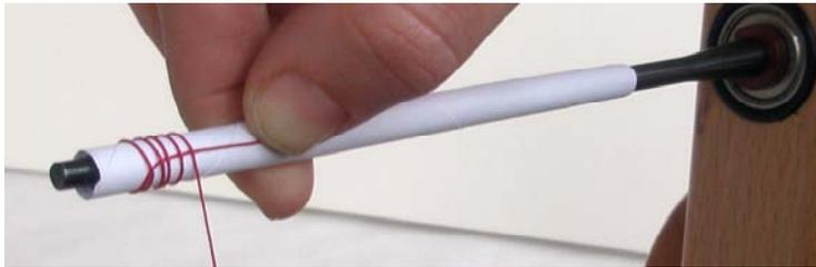
Using the hand crank, wind the bobbin winder (away from your body) and begin winding the thread around the quill. Use your other hand to guide the thread from the back of the quill (pulling from the spool rack), or guide from below (pulling from a cone).
