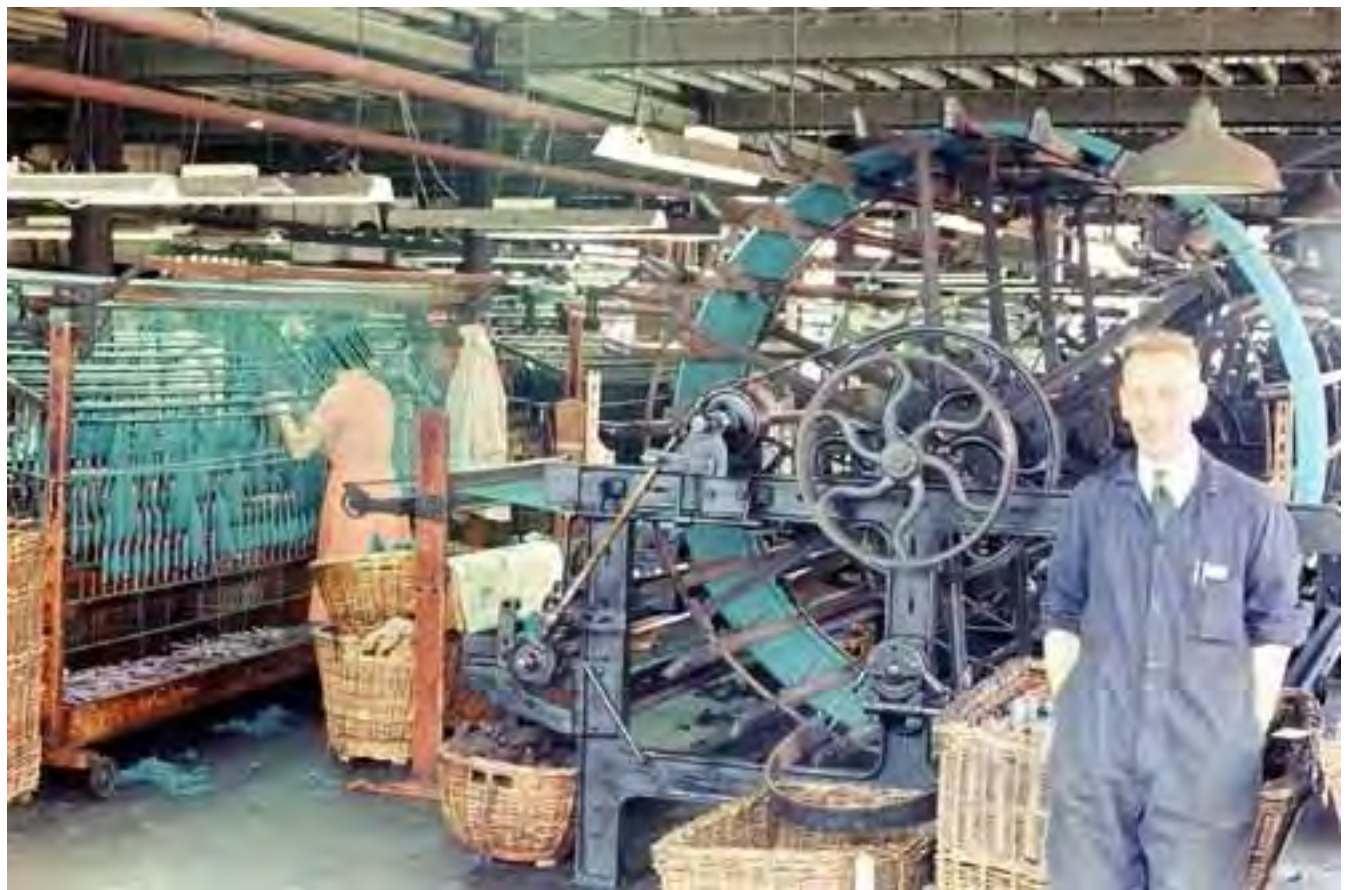
Wooden warping frame and balloon creel, Warping Department, Prospect Mills, Victoria Road, Cleckheaton, West Yorkshire, UK, 1965 http://www.leodis.net/display.aspx?resourceIdentifier=2006213_160695&DISPLAY=FULL
