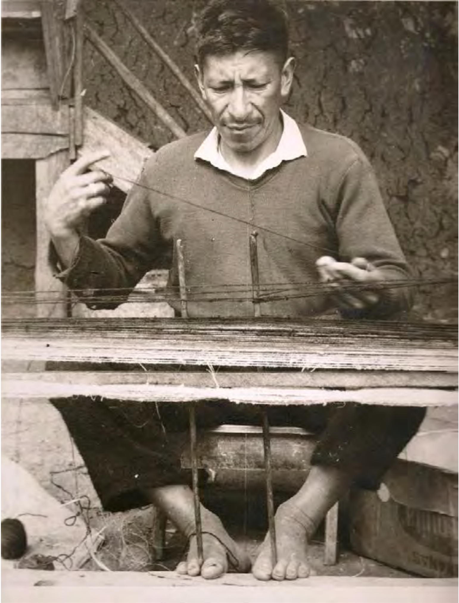
Circular warp being wound for a backstrap loom, Ecuador, 1960. Photo by Dennis Penley http://backstrapweaving.wordpress.com/2014/08/29/backstrap-weaving-fancy-footwork/
