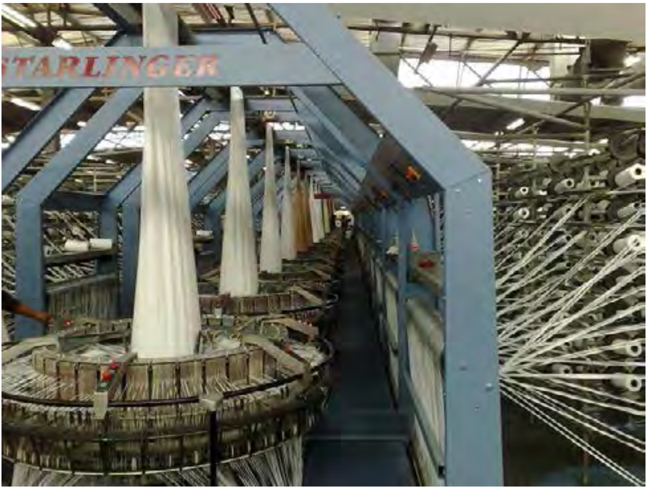
Polypropylene Bag Weaving and Warming Machine, 2012
