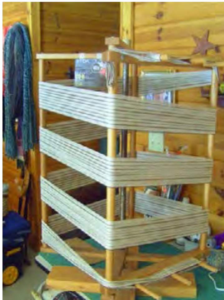
Warping reels used to wind the warp from Glimakra, Sweden. http://glimakrausa.com/glimakra-products/glimakra-warping-equipment/
